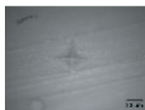
Indentation after firing at 760 °C for 2 min.* Surface is smoothed and hairline fractures are sealed.
